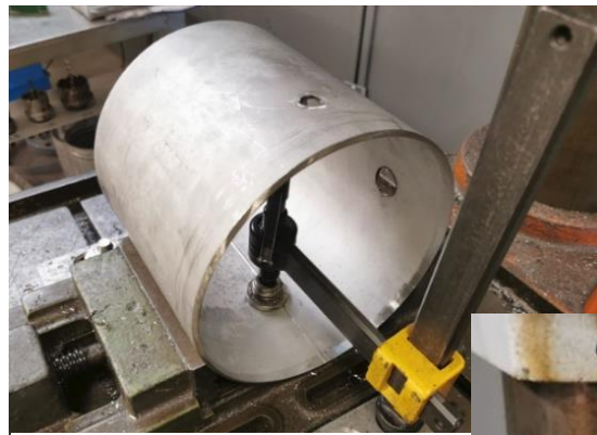
Figure 2 Properly secured pipe section
