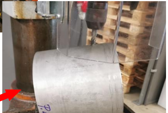
Figure 3 Piece of pipe after the drill bit has caught and pulled the workpiece upwards.
